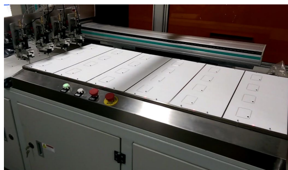
Antenna embedding for E-passport Inlay
