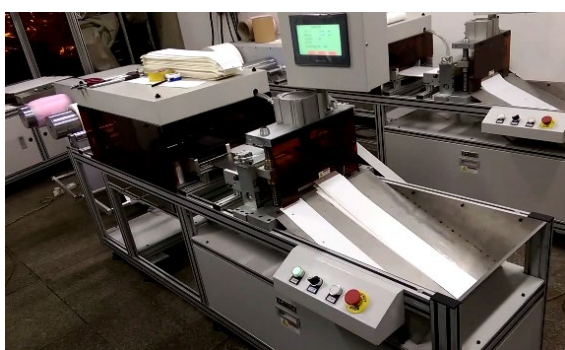
E-Passport Inlay roll Punching and Slitting (feeds in roll, punches positioning holes and chip holes in one go, and then slits)
